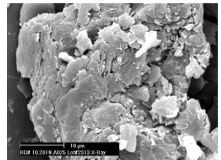
Below are two SEM images that illustrate the similarity between the micro-morphology of highly crystalline, naturally occurring flake graphite and finely ground synthetic graphite.
