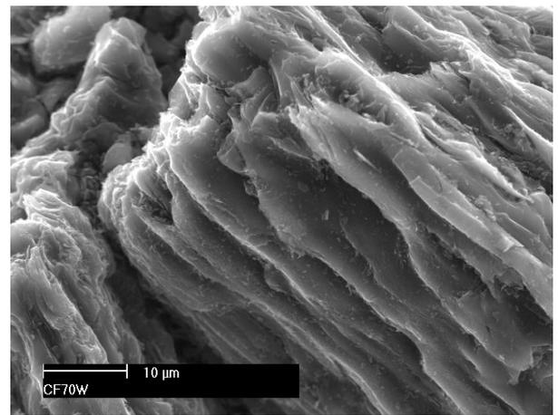
The micrograph on the left gives the viewer an indication of the gross morphology. The concentration of acicular coke visible in this material is very low, indicating an isotropic
