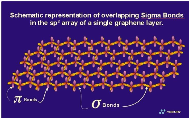
During the coking process (described elsewhere in this article) these layers form as the mesophase forms, grows, and organizes. These layer structures begin their existence as discotic (disk shaped) liquid crystals that coalesce into the mesophase.
